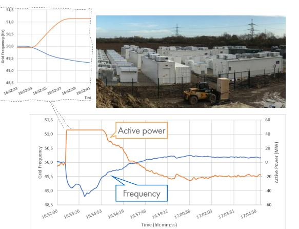
> Fast Frequency response products increase system stability, especially in grids with low inertia
