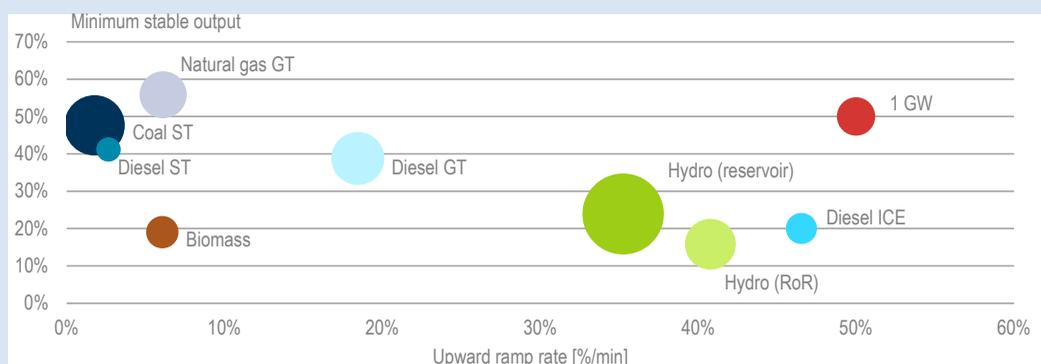
Notes: ST = steam turbine, GT = gas turbine, ICE = internal combustion engine, RoR = run of river, Nat = natural.
