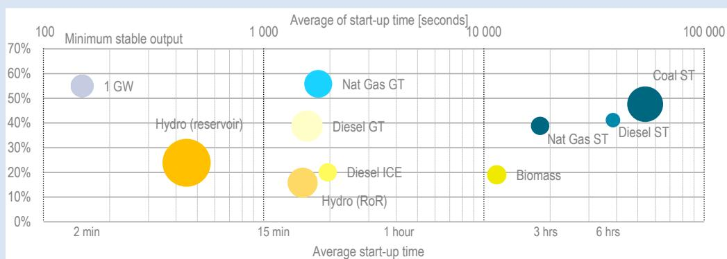
*Minimum stable output as a percentage of the nameplate capacity, upward ramp rate as a percentage of rated capacity per minute and capacity for selected technologies, 2015*
